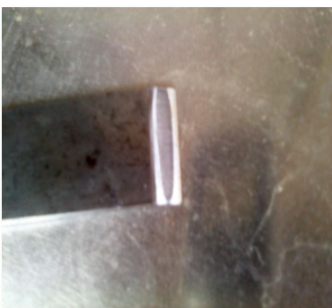
Fig. 3 Hollow Ground Chisel re-sharpened by Honing only
